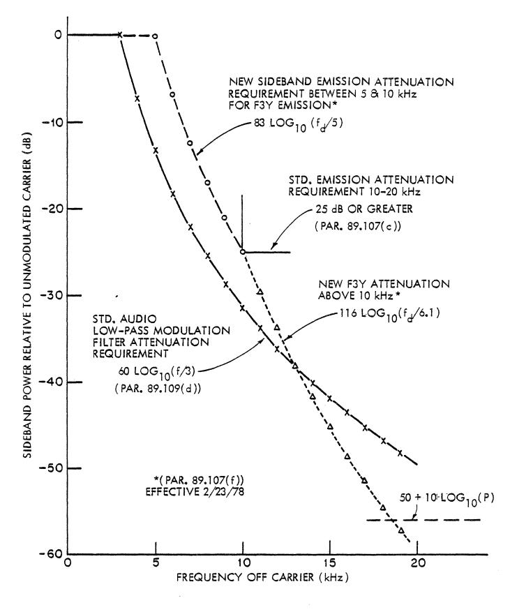
Fig. 30 Comparison of Standard Audio Low-Pass Filter and New Emission-Attenuation-Based Rolloff for F3Y Digital Modulation
