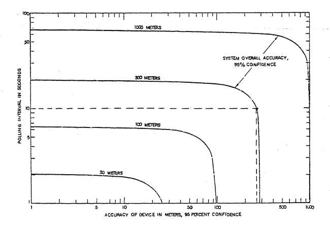
Figure 16 AVL System Accuracy versus Update Rate
