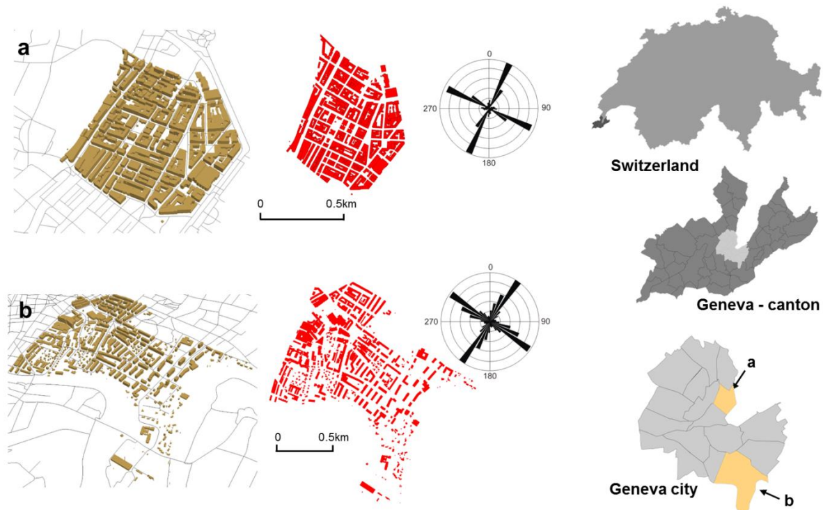
Fig. 2. Location of the city of Geneva in Switzerland and the 16 studied neighborhoods/zones of Geneva. A 3D view, a 2D (plan or map) view of the buildings, and the rose diagrams of the building orientations in (a) one of the old neighbourhoods/zones of Geneva (Paquis), (b) one of the more recent neighbourhoods/zones (Champel).
