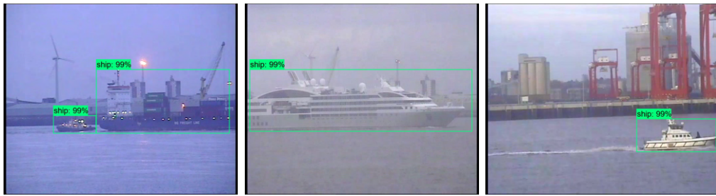
Figure 6.6: Example ship detections achieved using the developed Re-Trained SSD Inception v2 detector.
