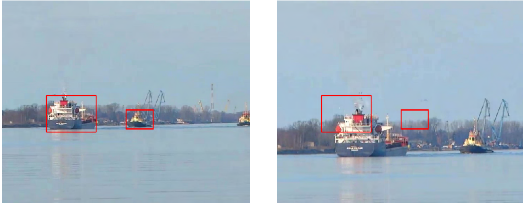
Figure 6.7: Example frames, along with annotated track estimates, before and after a camera command execution.
