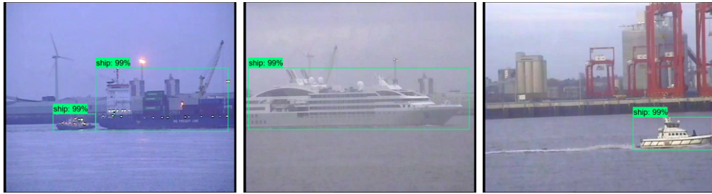
Figure 6.3: Samples extracted from the training and evaluation dataset. The ground truth annotations are depicted using green rectangles.
