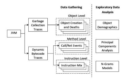
Figure 6.4: Schematic Diagram of Profiling Data Generation [117]
