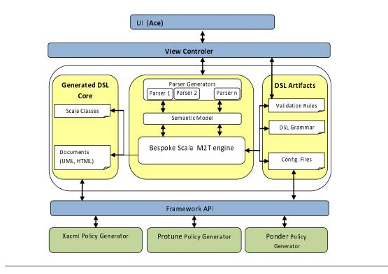
Figure 7.5: The Restructured Architecture of the Framework
