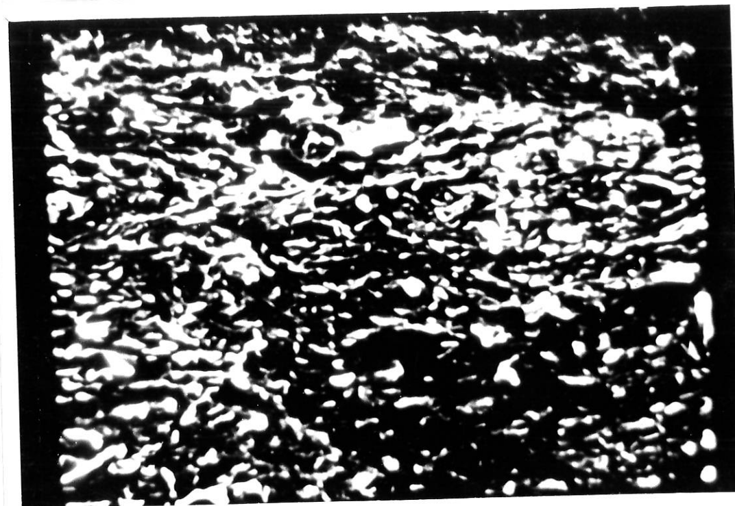
10 \mu\text{m} c) B2L 4.30 m, (unit 2, clay/gyttja transition). Horizontal clay flake fabric. Note the more compacted nature of the fabric, which may reflect greater compaction and dewatering at depth, but also the greater clay content of this unit. Scale bar = 10 \mu\text{m} .
