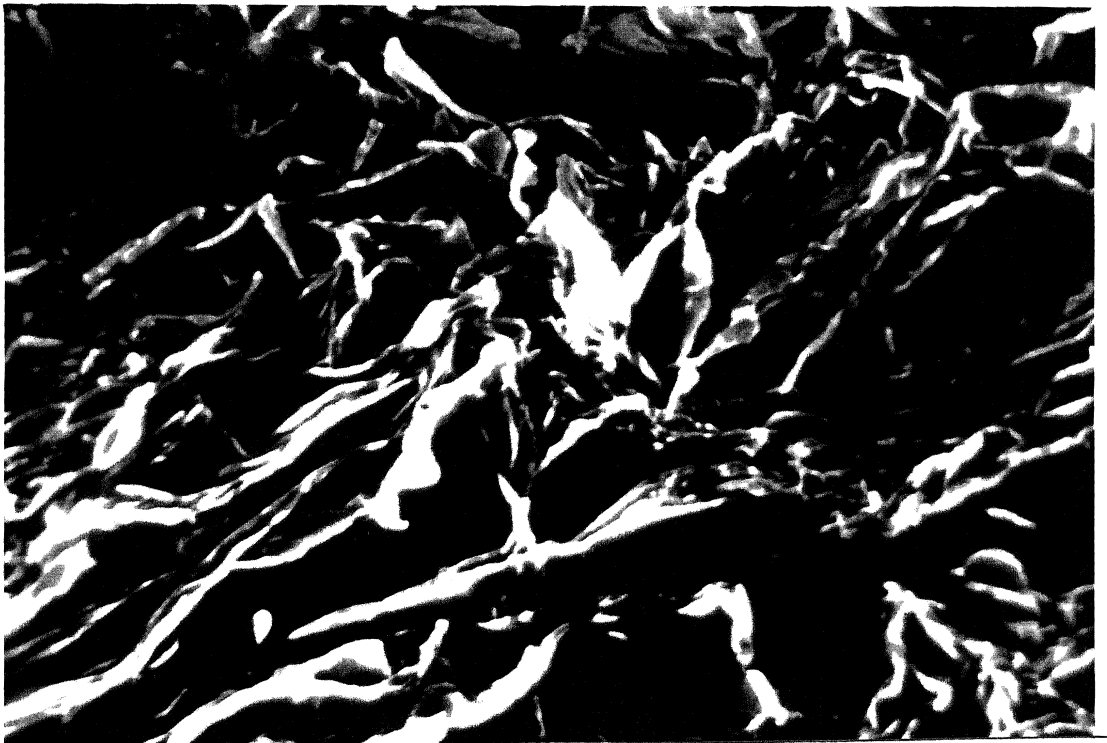
10 \mu\text{m} b) C2L 2.66 m. Severely disturbed or possibly primary random clay flake fabric. Fabric is still relatively compact in comparison to those from more organic-rich units. Scale bar = 10 \mu\text{m} .
