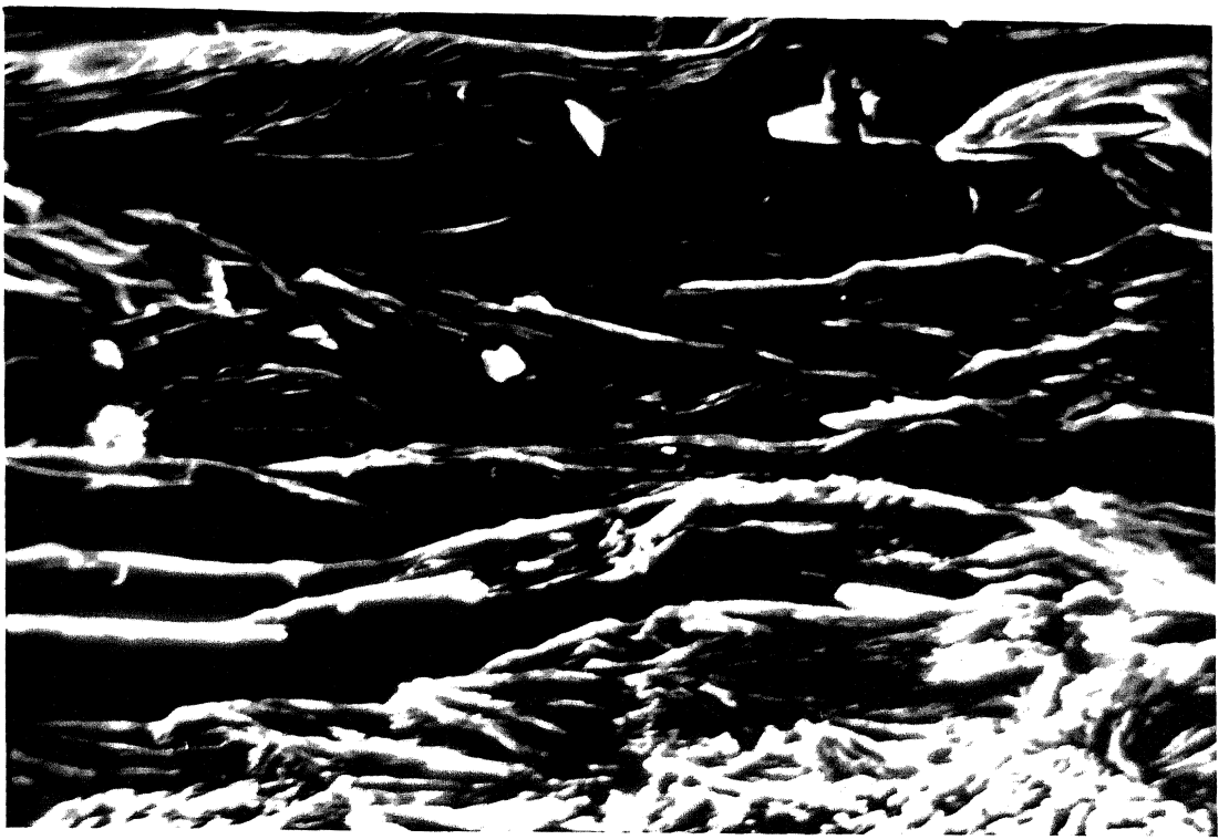
10 \mu\text{m} a) C2L 2.66 m. Horizontal clay flake fabric. Note the compactness of the fabric, particles stacked on top of one another. This reflects the platiness of the particles. Scale bar = 10 \mu\text{m} .
