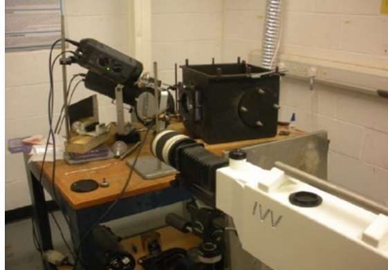
Figure 18. Expanding ring setup driven by detonation of explosive cap and associated diagnostics. From [164].
