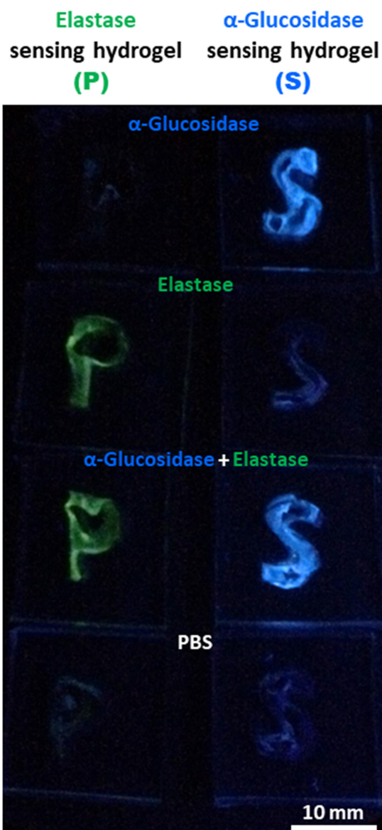
Figure 8. Photograph of the shape-encoded enzyme sensing hydrogels after enzymatic reactions. The photo was taken after a reaction time of 60 min under UV illumination (hand-held lamp, \lambda_{\text{ex}} = 365 \text{ nm} ) on a black background ( [\text{MUD}] = 1 \text{ mM} , [\text{ACS-HNE}] = 5 \text{ }\mu\text{M} , individual enzyme solutions [\alpha\text{-Glucosidase}] = 1.0 \text{ }\mu\text{M} , [\text{Elastase}] = 10 \text{ }\mu\text{M} were added in the 1 st and 2 nd row, respectively. A mixed enzyme solution ( [\alpha\text{-Glucosidase}] = 2.0 \text{ }\mu\text{M} , [\text{Elastase}] = 20 \text{ }\mu\text{M} with a volume ratio of 1:1) was applied in each letter patterns at the 3 rd row. PBS was added in the
