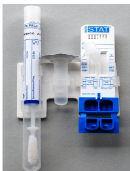
Figure 6. Mavand Rapid STAT ® saliva multi-drug test system (reproduced with permission from Elsevier [62]).
