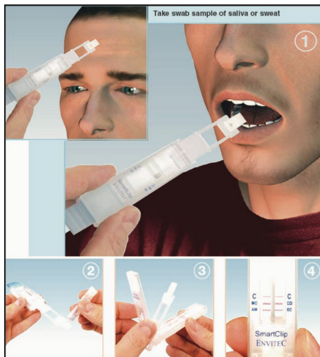
Figure 15. Smartclip device. (1) A swab of saliva or sweat is taken. (2) A buffer solution is added. (3) The system is closed. (4) The result can be read from indicator strips (reproduced with permission from Springer [51]).
