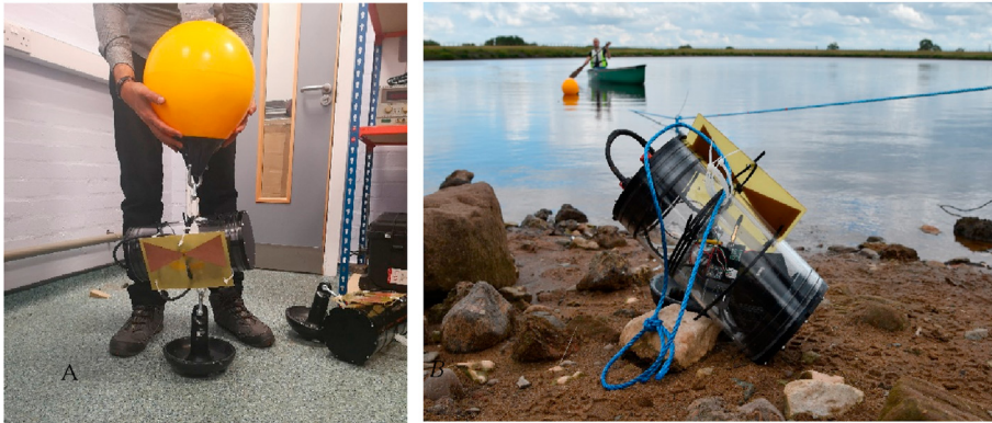
Fig. 6. (a) An example of the sensor node used during experimental works (b) An image of the experimental site where fieldwork was undertaken.
