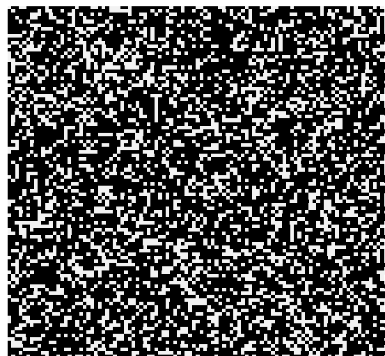
(d) p = 0.7 : The percolating cluster fills more space leaving less room for the smaller clusters
