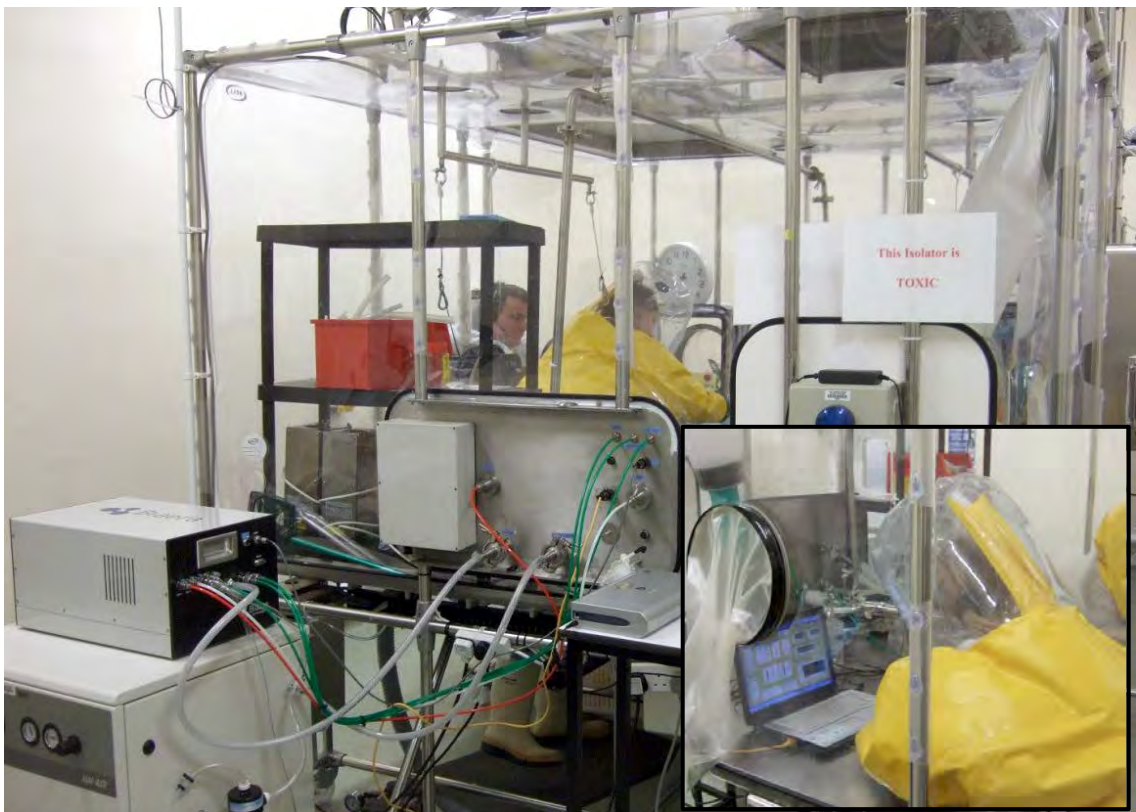
Figure 4 - A challenge isolator with the AeroMP-Henderson system. Insert displays the operator controlling the aerosol delivery from inside the isolator
