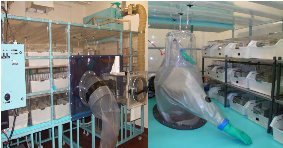
Figure 2 – Small Animal Flexible Film Isolator; shown with guinea pig caging
