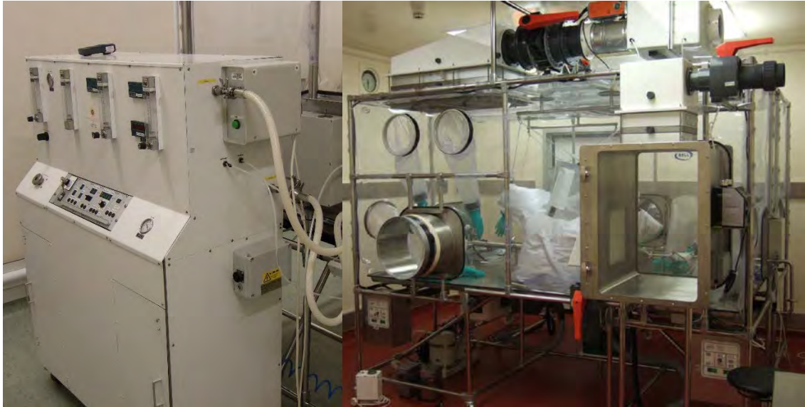
Figure 3 - An aerosol challenge isolator with the original mobile Henderson control
