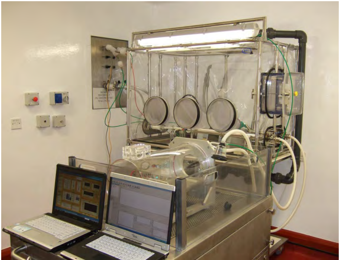
Figure 6 - AeroMP-Henderson NHP exposure system; Head-out plethysmography chamber and exposure mask
