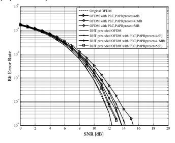
Fig.7. BER Performance of original OFDM signal and different techniques with SSPA over AWGN channel with 4-QAM modulation
