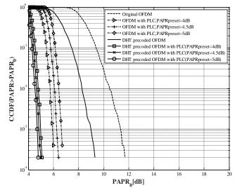
Fig.3. CCDFs of original OFDM signal and different PAPR reduction techniques with 4-QAM modulation
