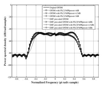
Fig.10. PSD's of original OFDM signal and different PAPR reduction techniques with 16-QAM modulation
