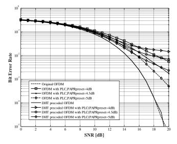
Fig.6. BER Performance of original OFDM signal and different techniques over AWGN channel with 16-QAM modulation
