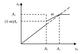
Fig.1. Piecewise linear companding transform
