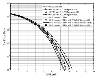
Fig.5. BER Performance of original OFDM signal and different techniques over AWGN channel with 4-QAM modulation
