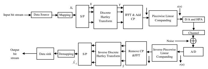
Fig.2. Block diagram of OFDM system with DHT and Piecewise Companding
