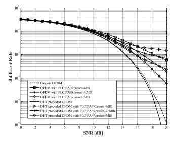
Fig.8. BER Performance of original OFDM signal and different techniques with SSPA over AWGN channel with 16-QAM modulation
