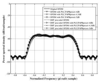
Fig.9. PSD's of original OFDM signal and different PAPR reduction techniques with 4-QAM modulation
