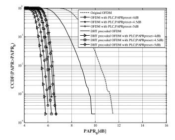
Fig.4. CCDFs of original OFDM signal and different PAPR reduction techniques with 16-QAM modulation
