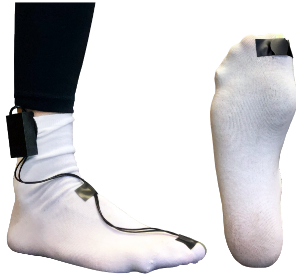
2 Fig. S1. Force sensors set-up. Force sensors are taped underneath the big toes of the user's feet and 4 powered by the external batteries strapped around the ankles. Pressure exerted with the right toe 6 controls flexion of the Thumb while the pressure exerted with the left toe controls the abduction. The extent of Thumb movement is fully proportional to the pressure applied. As such the Thumb can be used when sitting or standing, but not while walking.
