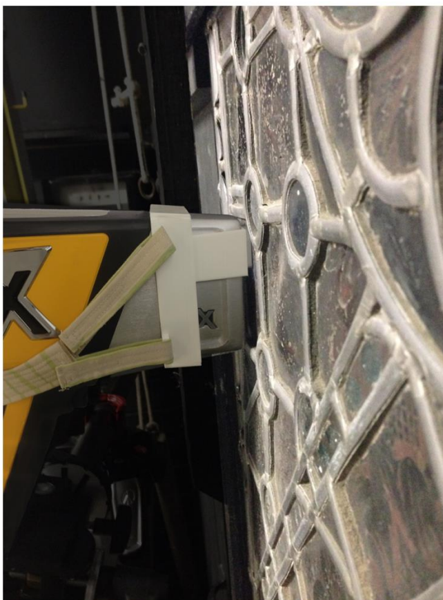
Figure X-5 A window analyzer attachment nicknamed the WindoLyzer 5 was designed using tinkercad.com (top left) and 3D printed at the Institute of Making at UCL. The attachment is secured to the spectrometer using Velcro on a fabric strap (bottom left) and used to analyze the Methuselah panel from Canterbury Cathedral (right).
