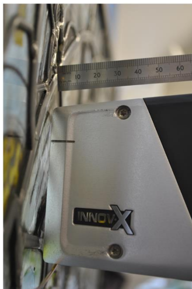
Figure X-2 Lead comes can protrude multiple millimeters, and together with the use of small pieces of glass, prohibit the placement of the pXRF spectrometer directly on the surface of the glass for analysis. The panel in this image has been recently conserved and releaded, and the modern lead comes in these panels protrude by about 2-4mm.
