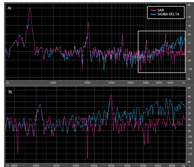
Figure 5. Comparing of frequency of bird voices by two types of A/D converters
