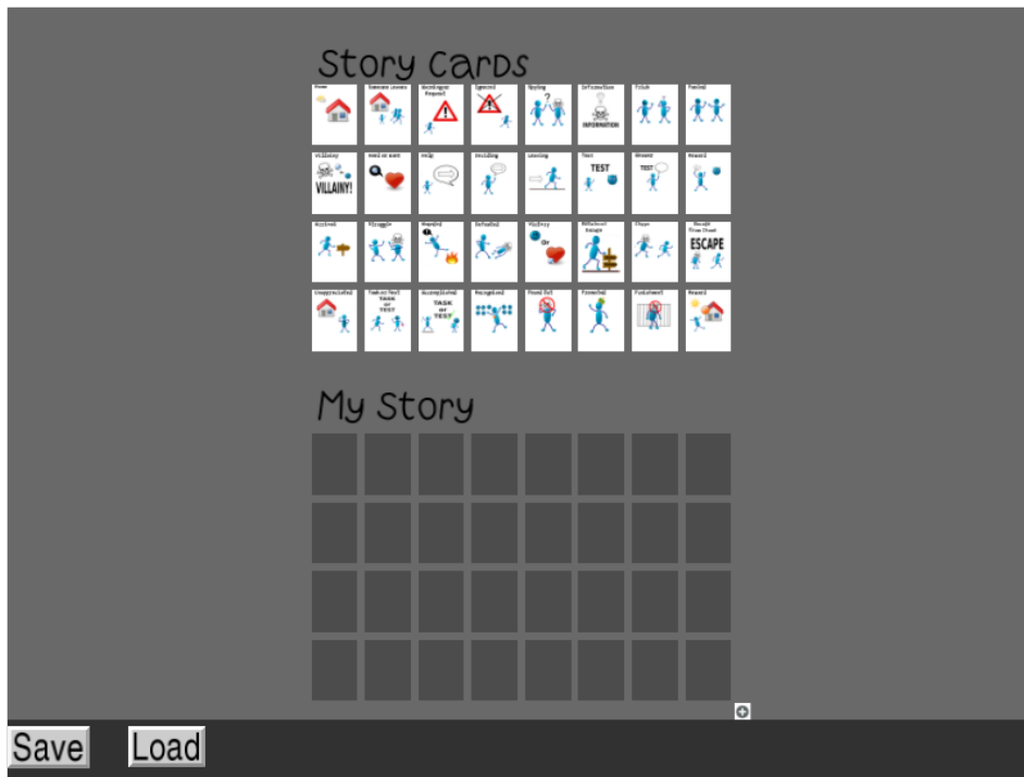
Figure 5.9: A screenshot of the prototype story maps application with the toolbar in view at the bottom of the screen. The toolbar slides into view when the user moves the mouse pointer to the bottom edge of the screen, and slides out of view again when the user moves the mouse pointer away.
