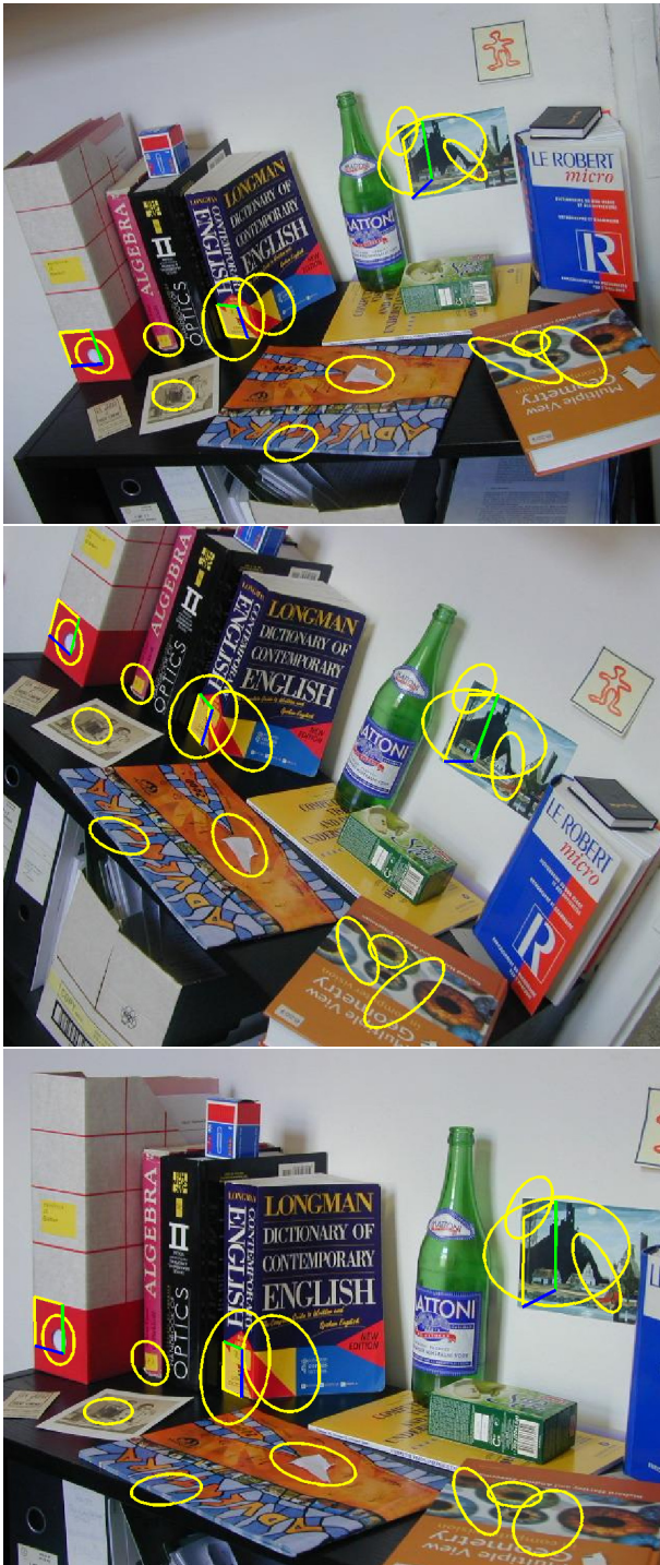
Figure 4: The features that could be matched in each of the 3 views of fig. 3. This intersection of the pairwise matching sets is quite small: only 16 features remain.
