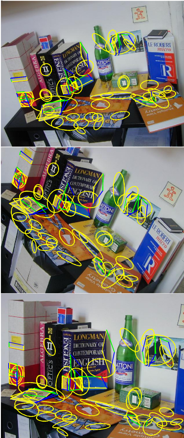
Figure 5: The features that could be matched in each of the 3 views of fig. 4 after propagation and transitivity reasoning. The number of matches has been increased to 58.
