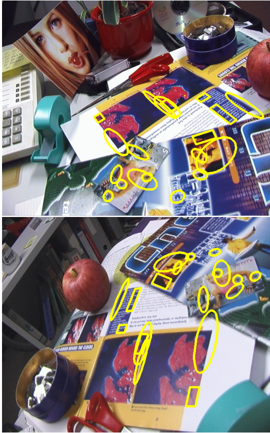
Figure 2: ‘invariant neighbourhoods’ that were extracted for the images in fig. 1. Only regions are shown for which a corresponding partner in the other image has been found, but the regions in the two images have been extracted without knowledge about the other image.
