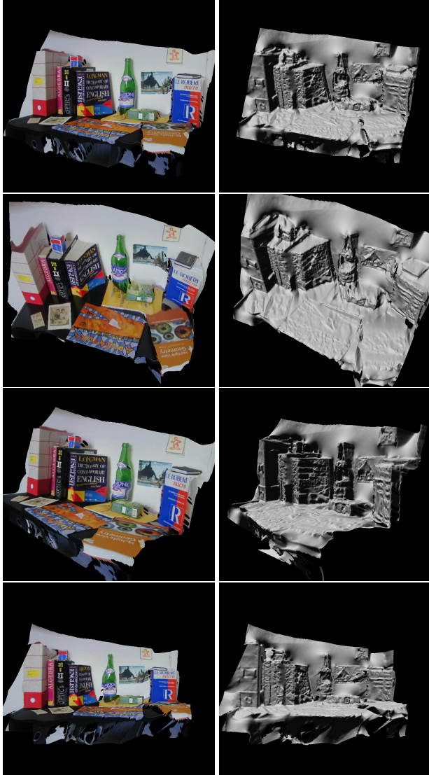
Figure 7: Textured and untextured views of the dense reconstruction of the bookshelf scene shown in figure 3. The images are too far apart for our traditional shape-from-video pipeline to match.
