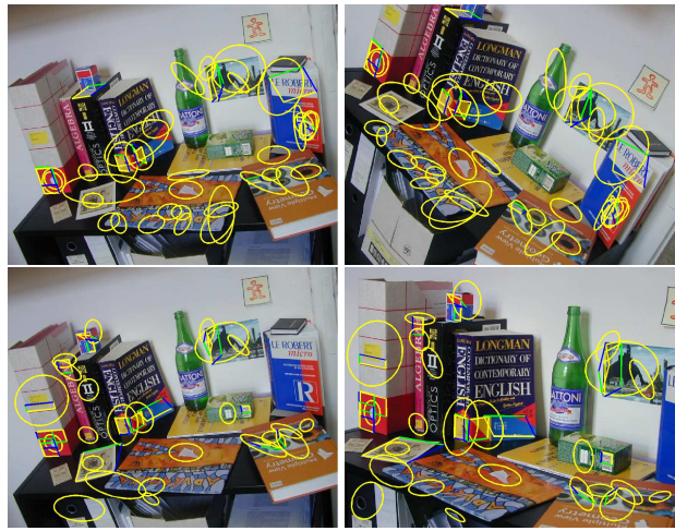
Figure 4: Three wide-baseline views of the ‘bookshelf’ scene. The top two images show image 1 and 2 with the corresponding invariant regions. The bottom two images show the same for image 1 and 3.
