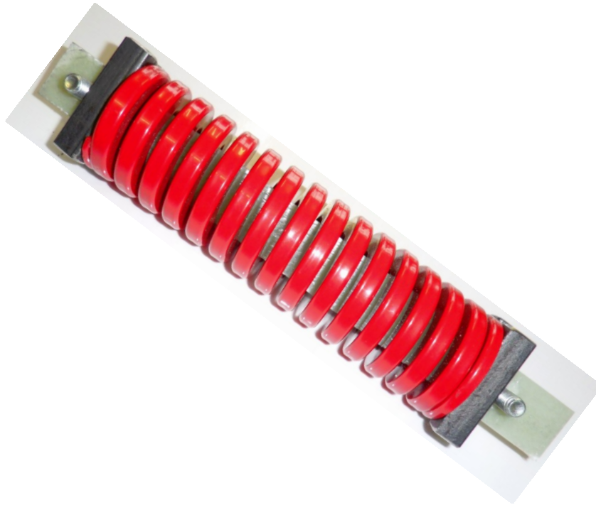
Figure 3. Stressing mechanism for stress ageing of GFRP coupon.
