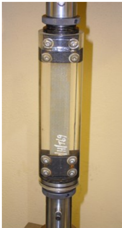
Figure 4. Immersed fatigue test setup, acrylic tube with O-ring seal.
