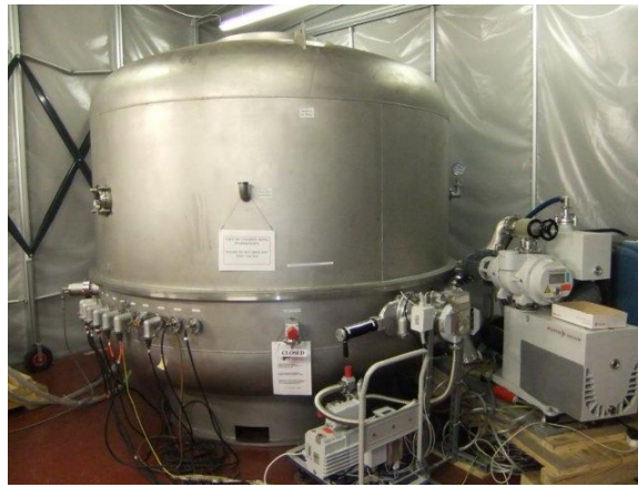
(c) Vacuum chamber with helium cryocoolers [12].
