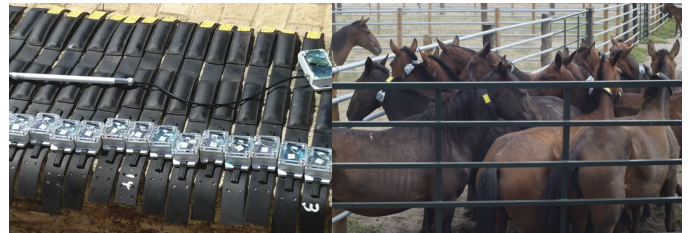
Fig. 1. An arrangement of mobile nodes with a base-station and antenna ready for deployment (left). Wild horses being marked with sensors (right).
