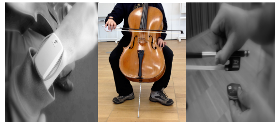
Figure 1: Cellist (Centre) with an Orient Speck attached to the wrist (Left) and another one attached to the frog of the bow (Right).
