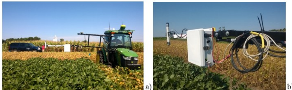
Figure 14a. Piccolo Doppio with OO USB 2000+ and NIRQuest on tractor and b) Up- and down-welling fore optics on gimbal. Photos provided by A. Singh, U. of Wisconsin)
