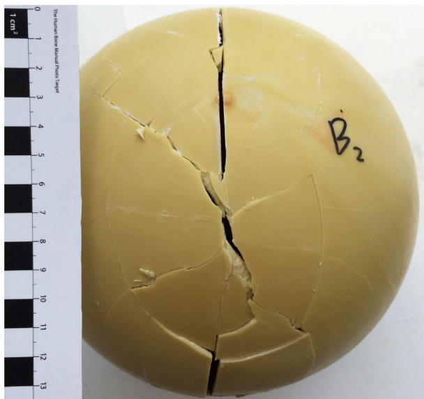
Figure 6 Depressed fracture on SYNBONE sphere filled with porcine gelatin simulating a free-moving head after strike with a baseball bat. Photograph courtesy of Yi-Hua Tang.
