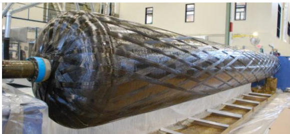
Fig. 1. Vessel of carbon fibre composite during manufacturing
