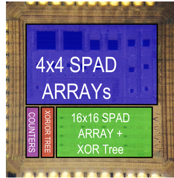
Figure 4. Test Chip - A selected samples of dSiPMs has been manufactured on the same test chip. All the varieties of dSiPMs have been combined through toggle cells and a common XOR tree outside the cells.
