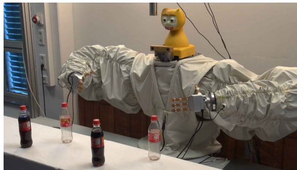
Figure 5: In the BIMANUAL scenario, a camera is used to recognise empty bottles which a bimanual robot should remove from to a “dishwasher” location on the left side, behind the table (Gaschler et al. 2013a; Giuliani et al. 2013).
