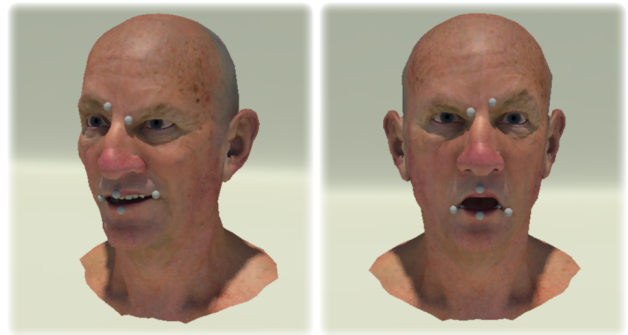
Figure 9: Application to facial model in a FaceIK fashion. The user moves the control points and the rig parameters of the face are computed to satisfy the constraints.
