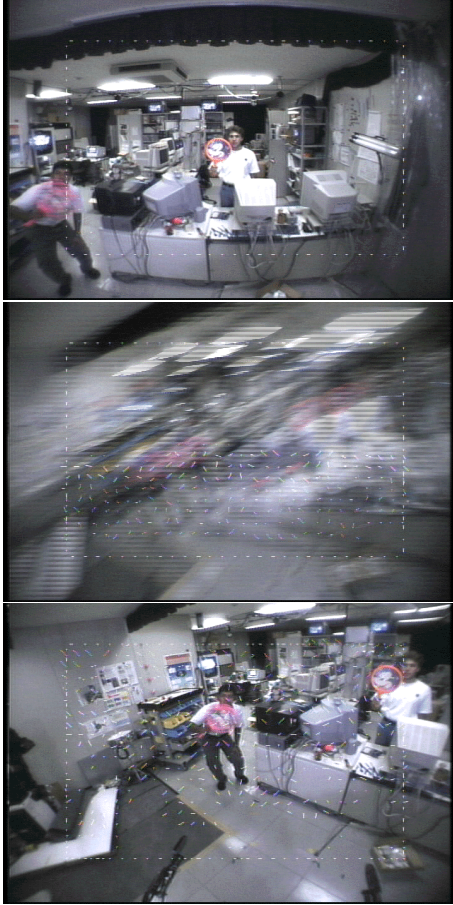
Figure 8: Snap shots of the robot’s peripheral view before, during, and after an attentional head-eye saccade, taken at 30 Hz sampling rate. Superimposed on the images is the visual flow field.
