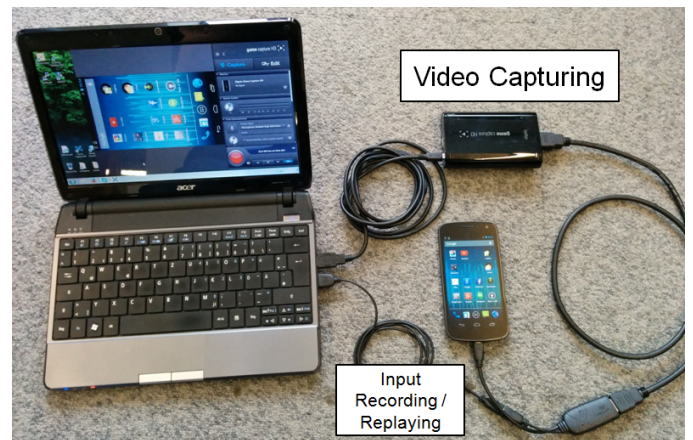
Fig. 6. We capture a video of the mobile screen output by recording an HDMI signal with a video capture device like the Elgato Game Capture HD [7].
