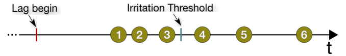
Fig. 9. This figure shows the timeline of a single interaction lag. Each circled number stands for the lag ending of a specific system configuration. Each lag length that stays below the specified Irritation Threshold does count as not irritating and for each lag length that exceeds it a penalty is applied.
