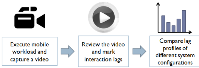
Fig. 1. Execute an interactive workload and record screen output in a video. Automatically identify interaction lag timings in the video and evaluate them in terms of user satisfaction.
