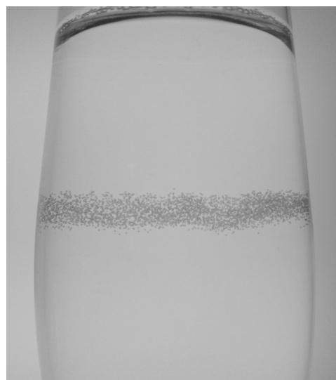
FIG. 1. Photograph of nucleation of carbon dioxide bubbles caused by passage of the laser pulse (5 ns pulse duration) from left to right. For illustration purposes, a high laser power ( \sim 60 MW cm ^{-2} ) was used to create many bubbles.
