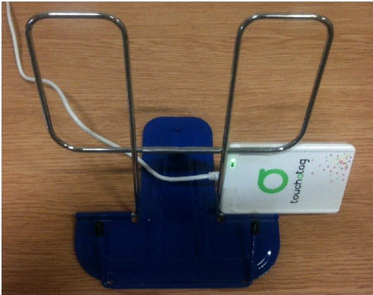
Figure 2: A book stand with a 'Touchatag' RFID sensor attached to the bottom right section.
