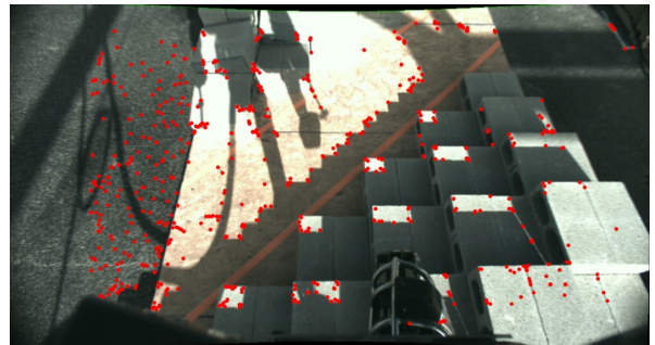
Fig. 8. In realistic field scenarios such as the DRC Trials, strong shadows and self observations result in false visual features (shown in red).
