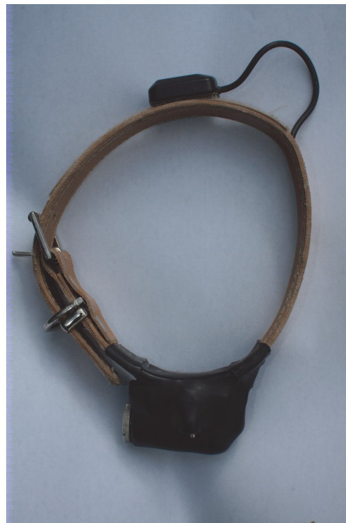
Fig 1. The GPS collar. The battery compartment, GPS and logger with external toggle switch all positioned ventrally and a movable GPS antenna located dorsally.
