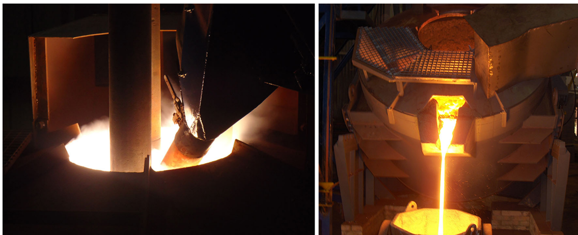
Fig. 4 Photos of the EAF during batch feeding ( left ) and during pouring ( right )
