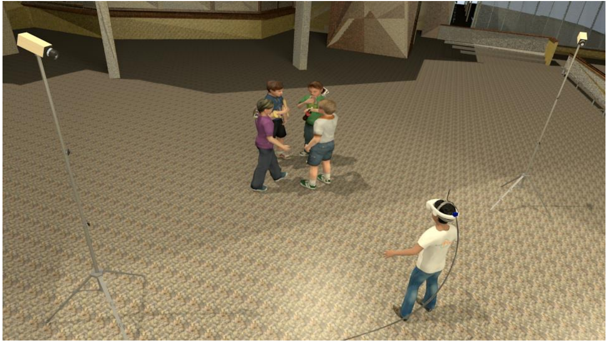
Figure 1. Schematic representation of the virtual reality setup. The participant (lower right-hand corner) viewed the virtual environment wearing an nVisor SX60 stereoscopic head-mounted display (HMD) with a resolution of 1280x1024 and a diagonal field of view of 60 degrees in each eye. Head rotations were tracked using an InertiaCube3 three-axis orientation tracker attached to the head-mounted display. A LED marker on top of the HMD signaled the participant's position in the virtual environment to a system (Precision Position Tracking, PPT X) of four optical cameras mounted on tripods in each corner of the lab (two shown at the left- and right-hand). The orientation and position information gathered was transferred to the rendering machine via HMD and camera cables to update the graphics displayed in the HMD. The avatars (Vizard Complete Characters) were placed in a 3D model of a schoolyard around 7 meters in front of the participant.
