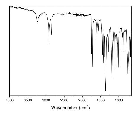
**Figure S50.** FT-IR spectrum of diethyl 4-(dodecyloxy)pyridine-2,6-dicarboxylate (dpaC<sub>12</sub>H<sub>25</sub>). IR (cm<sup>-1</sup>) 3240, 2918, 2850, 1753, 1734, 1725, 1604, 1562, 1466, 1445, 1417, 1402, 1362, 1279l, 1190, 1106, 1055, 1031, 1010, 907, 877, 754, 695, 681, 639, 614.
