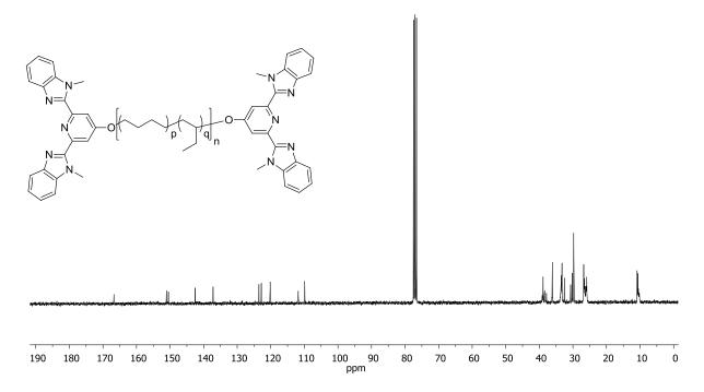
**Figure S39.** <sup>13</sup> C NMR spectrum of the BKB macromonomer.<sup>13</sup>C NMR (75 MHz, CDCl<sub>3</sub>): δ 166.59, 151.27, 150.31, 142.64, 137.20, 123.63, 122.89, 120.17, 112.05, 109.82, 68.56, 38.40-37.83, 35.96, 33.49, 33.24, 32.53, 30.66, 30.21, 29.77, 26.78-25.88, 10.83-10.18.
