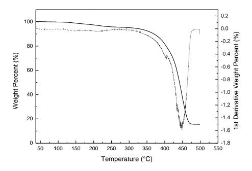
**Figure S8.** Thermal analysis of  $[Eu(DKD)_{1.5}](NHEt_3)_3$ . Thermogravimetric analysis (TGA) curves of  $[Eu(DKD)_{1.5}](NHEt_3)_3$  from 25 to 500 °C; weight percent (—) and derivative weight percent (…). The experiment was conducted at a heating rate of 10° C/min under N<sub>2</sub> atmosphere.
