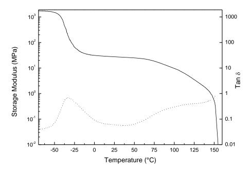
**Figure S1.** Mechanical analysis of  $[Eu(BKB)_{1.5}](ClO_4)_3$ . Representative dynamic mechanical thermal analysis (DMTA) traces of  $[Eu(BKB)_{1.5}](ClO_4)_3$  (ca. 200 µm thickness) from -70 to 160 °C; storage modulus (—) and tan  $\delta$  (…). Experiments were conducted under N<sub>2</sub> atmosphere at a heating rate of 3 °C/min and a frequency of 1 Hz. At 25 °C, the storage modulus is  $23 \pm 6$  MPa.
