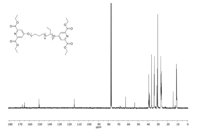
**Figure S44.** <sup>13</sup>C NMR spectrum of the ethyl protected DKD macromonomer. <sup>13</sup>C NMR (CDCl<sub>3</sub>, 90 MHz) δ 167.09, 165.28, 164.77, 150.10, 149.75, 114.60, 114.49, 114.36, 62.38, 53.12, 39.10, 38.87, 38.40, 37.89, 36.12, 33.44, 33.24, 30.66, 30.21, 29.75, 26.78, 26.60, 26.44, 26.26, 26.13, 26.04, 25.88, 14.19, 10.88, 10.68, 10.64, 10.53, 10.35, 10.21.
