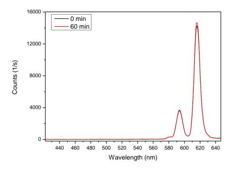
**Figure S35.**Photoluminescence spectra of  $[Eu(DKD)_{1.5}](NHEt_3)_3$  polymer films. Thin films of  $[Eu(DKD)_{1.5}](NHEt_3)_3$  were swollen in a solution of  $Fe(ClO_4)_2$  in CH<sub>3</sub>CN (10 mL, 0.5 mM) for 5 days and then ultrasonicated in the same solution for 1 h (0.5 sec pulse, 1 sec delay). The emission spectra were recorded before (black line) and after this process (red line) using a fiber optic cable and excitation with a handheld UV lamp ( $\lambda = 254$  nm).
