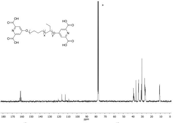
**Figure S46.** <sup>13</sup>C NMR spectrum of the DKD macromonomer.<sup>13</sup>C NMR (75 MHz, CDCl<sub>3</sub>) δ 77.16, 39.05, 36.29, 33.61, 33.41, 30.83, 30.38, 29.93, 26.95, 26.76, 26.61, 26.29, 26.21, 26.05, 11.02, 10.80.
