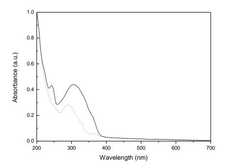
**Figure S28.** Solid-state UV-vis absorption spectra of the metallopolymers. UV-Vis absorption spectra acquired for drop-cast thin films from a CHCl<sub>3</sub> solution (0.8 mg/mL, 125  $\mu$ L): [Eu(BKB)<sub>1.5</sub>](ClO<sub>4</sub>)<sub>3</sub> ((—), 3  $\mu$ m thick) and [Eu(DKD)<sub>1.5</sub>](NHEt<sub>3</sub>)<sub>3</sub>((···), 1.4  $\mu$ m thick).
