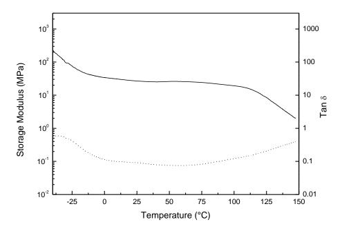
**Figure S32.** Mechanical analysis of  $[Fe(BKB)](ClO_4)_2$ . Representative dynamic mechanical thermal analysis (DMTA) traces of  $[Fe(BKB)](ClO_4)_2$  (ca. 200 µm thickness) from -40 to 150 °C; storage modulus (—) and tan  $\delta$  (…). Experiments were conducted under N<sub>2</sub> atmosphere at a heating rate of 3 °C/min and a frequency of 1 Hz. At 25 °C, the storage modulus is  $26 \pm 1$  MPa.
