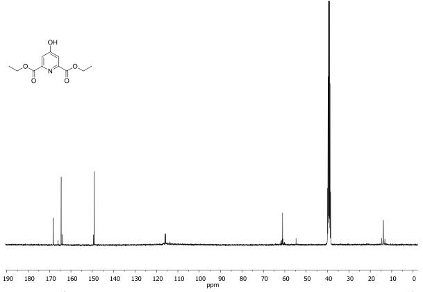
**Figure S42.** <sup>13</sup>C NMR spectrum of 4-hydroxy-pyridine-2,6-dicarboxylic acid diethyl ester.<sup>13</sup>C NMR (90 MHz, DMSO-*d*6) δ 168.85, 165.08, 149.57, 116.60, 116.28, 61.58, 14.50, 14.42.
