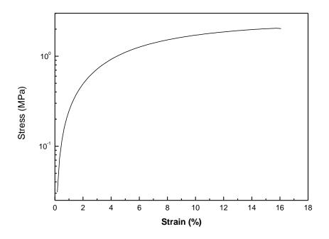
**Figure S3.** Mechanical analysis of  $[Eu(BKB)_{1.5}](ClO_4)_3$ . Representative stress-strain curve of  $[Eu(BKB)_{1.5}](ClO_4)_3$ . Measurements were conducted under N<sub>2</sub> atmosphere at 25 °C, with a strain rate of 5%/min.
