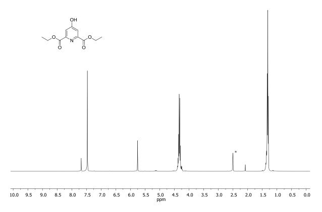
**Figure S41.** <sup>1</sup>H NMR spectrum of 4-hydroxy-pyridine-2,6-dicarboxylic acid diethyl ester. <sup>1</sup>H NMR (360 MHz, DMSO-*d*6)  $\delta$  7.47 (s, 2H, Ph-*H*), 5.75 (s, 1H, C-O*H*), 4.32 (q, *J* = 7.1 Hz, 4H, -O-CH<sub>2</sub>-CH<sub>3</sub>), 1.31 (t, *J* = 7.2 Hz, 6H, -O-CH<sub>2</sub>-CH<sub>3</sub>).
