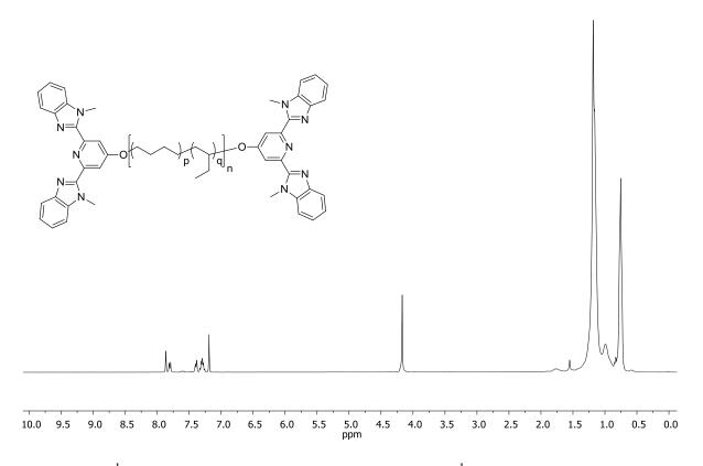
**Figure S38.** <sup>1</sup>H NMR spectrum of the BKB macromonomer. <sup>1</sup>H NMR (360 MHz, CDCl<sub>3</sub>):  $\delta$  7.93 (s, 4H), 7.86 (d, *J* = 7.8 Hz, 4H), 7.45 (d, J = 7.8 Hz, 4H), 7.37 (m, 8H), 4.24 (broad s, 16H), 1.25 (m, 437 H), 0.82 (m, 152H).
