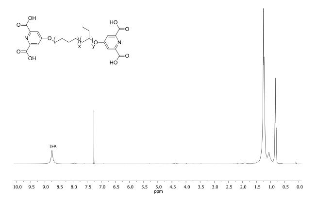
**Figure S45.** <sup>1</sup>H NMR spectrum of the DKD macromonomer. <sup>1</sup>H-NMR (CDCl<sub>3</sub>/TFA (30:1), 300 MHz):  $\delta$  8.00 (s, 4H), 4.42 (s, 4H), 2.22 – 0.97 (m, 561H), 0.83 (t, *J* = 6.8 Hz, 180H).
