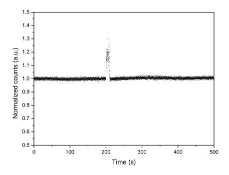
**Figure S22.** *In situ* monitoring of ultrasound induced changes of the neat BKB monomer by photoluminescence spectroscopy. A solution of BKB in  $CHCl_3$  (2.0 mg/ml) was subjected to one sonication pulse with a duration of 10 sec. The solution was excited at 347 nm and the emission was monitored at 440 nm.
