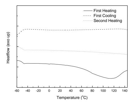
**Figure S6.** Thermal analysis of  $[Eu(DKD)_{1.5}](NHEt_3)_3$ . Modulated differential scanning calorimetry (DSC) curves of  $[Eu(DKD)_{1.5}](NHEt_3)_3$ ; first heating (—), first cooling (- - ) and second heating (…). The experiment was conducted with heating and cooling rates of 10° C/min under N<sub>2</sub> atmosphere.
