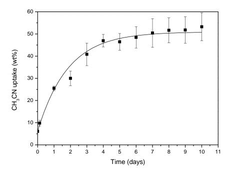
**Figure S29.** Swelling behavior of  $[Eu(BKB)_{1.5}](ClO_4)_3$ . Thin films of  $[Eu(BKB)_{1.5}](ClO_4)_3$  were placed in CH<sub>3</sub>CN for up to 10 days at room temperature. The degree of swelling was determined by measuring the weight of the samples pre- and post-swelling. Data points represent averages (number of individual measurements, n = 3) ± standard deviation.
