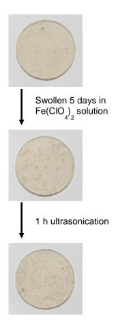
**Figure S34.** Images of  $[Eu(DKD)_{1.5}](NHEt_3)_3$  swollen and ultrasonicated in  $Fe(ClO_4)_2$  solution. Thin films of  $[Eu(DKD)_{1.5}](NHEt_3)_3$  were swollen in a solution of  $Fe(ClO_4)_2$  in CH<sub>3</sub>CN (10 mL, 0.5 mM) for 5 days and then ultrasonicated in the same solution for 1 h (0.5 sec pulse, 1 sec delay).
