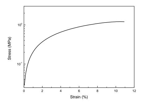
**Figure S4.** Mechanical analysis of  $[Eu(DKD)_{1.5}](NHEt_3)_3$ . Representative stress-strain curve of  $[Eu(DKD)_{1.5}](NHEt_3)_3$ . Measurements were conducted under N<sub>2</sub> atmosphere at 25 °C, with a strain rate of 5%/min.
