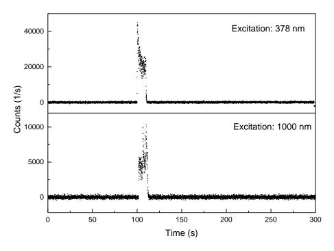
**Figure S21.** Sonoluminescence of CHCl<sub>3</sub>. CHCl<sub>3</sub> was subjected to one ultrasonication pulse with a duration of 10 sec. The solution was excited at various wavelengths (top:  $\lambda_{ex} = 375$  nm; bottom:  $\lambda_{ex} = 1000$  nm) and the emission was monitored at 615 nm. The response was found to be independent of the excitation wavelength.
