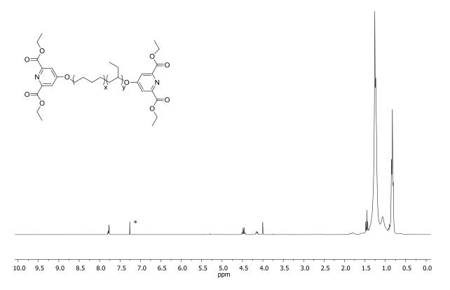
**Figure S43.** <sup>1</sup>H NMR spectrum of the ethyl protected DKD macromonomer. <sup>1</sup>H-NMR (CDCl<sub>3</sub>, 300 MHz)  $\delta$  7.79 (s, 4H), 4.49 (q, 5H), 4.16 (q, *J* = 6.8 Hz, 4H), 4.02 (s), 1.93 – 0.96 (m, 510H), 1.47 (t, *J* = 7.1 Hz, 7H), 0.84 (t, *J* = 6.8 Hz, 157H). Small impurities at 4.02 ppm originating from DIAD, and partial deprotection of carboxylic acid were observed.
