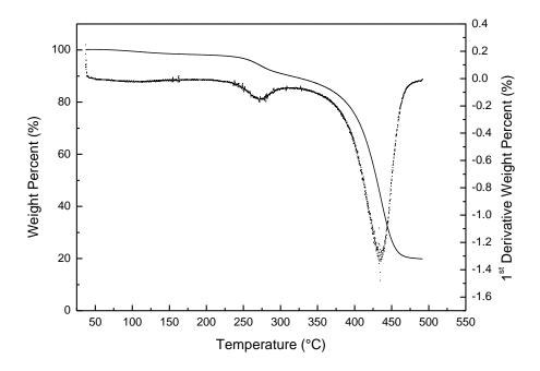
**Figure S7.** Thermal analysis of  $[Eu(BKB)_{1.5}](ClO_4)_3$ . Thermogravimetric analysis (TGA) curves of  $[Eu(BKB)_{1.5}](ClO_4)_3$  from 25 to 500 °C; weight percent (—) and derivative weight percent (…). The experiment was conducted at a heating rate of 10° C/min under N<sub>2</sub> atmosphere.
