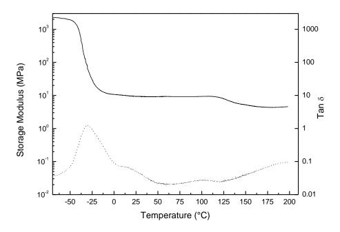
**Figure S2.** Mechanical analysis of  $[Eu(DKD)_{1.5}](NHEt_3)_3$ . Representative dynamic mechanical thermal analysis (DMTA) traces of  $[Eu(DKD)_{1.5}](NHEt_3)_3$  (ca. 200 µm thickness) from -70 to 200 °C; storage modulus (—) and tan  $\delta$  (…). Experiments were conducted under N<sub>2</sub> atmosphere at a heating rate of 3 °C/min and a frequency of 1 Hz. At 25 °C, the storage modulus is 8 ± 1.5 MPa.
