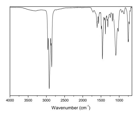
**Figure S51.** FT-IR spectrum of metallosupramolecular polymer [Eu(BKB)<sub>1.5</sub>](ClO<sub>4</sub>)<sub>3</sub>.IR (cm<sup>-1</sup>) 3309, 2959, 2921, 2872, 2852, 1719, 1606, 1566, 1491, 1460, 1407, 1379, 1330, 1312, 1243, 1187, 1093, 1026, 930, 866, 754, 747, 723, 622.
