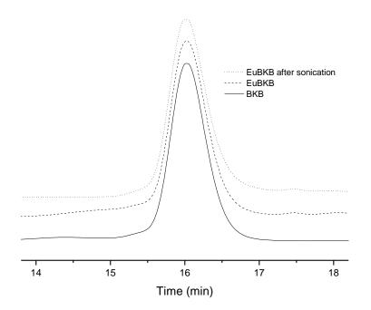
**Figure S37.** Gel permeation chromatography (GPC) traces of BKB and  $[Eu(BKB)_{1.5}](ClO_4)_3$  in THF. Samples of BKB (solid line) and  $[Eu(BKB)_{1.5}](ClO_4)_3$  (dash line) were analyzed by GPC before ultrasonication. Films of  $[Eu(BKB)_{1.5}](ClO_4)_3$  were ultrasonicated for 1 h (0.5 sec pulse, 1 sec delay) and then dried in vacuum. Ultrasonicated  $[Eu(BKB)_{1.5}](ClO_4)_3$  films (dotted line) were then dissolved in THF and analyzed by GPC.
