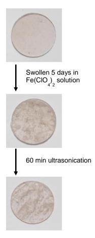
**Figure S36.** Images of  $[Zn(BKB)_{1.0}](ClO_4)_2$  swollen and ultrasonicated in Fe(ClO<sub>4</sub>)<sub>2</sub> solution. Thin films of  $[Zn(BKB)_{1.0}](ClO_4)_2$  were swollen in a solution of Fe(ClO<sub>4</sub>)<sub>2</sub> in CH<sub>3</sub>CN (10 mL, 0.5 mM) for 5 days and then ultrasonicated in the same solution for 1 h (0.5 sec pulse, 1 sec delay).
