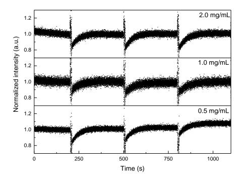
**Figure S16.** In situ monitoring of the ultrasound induced dissociation of  $[Eu(BKB)_{1.5}](ClO_4)_3$ by photoluminescence spectroscopy. Solutions of  $[Eu(BKB)_{1.5}](ClO_4)_3$  in CHCl<sub>3</sub> (2.0, 1, or 0.5 mg/ml) were subjected to three sonication pulses with a duration of 10 sec each. The samples were excited at 375 nm and the intensity of the Eu<sup>3+ 5</sup>D<sub>0</sub>  $\rightarrow$  <sup>7</sup>F<sub>2</sub> emission band was monitored at 615 nm as a function of time.
