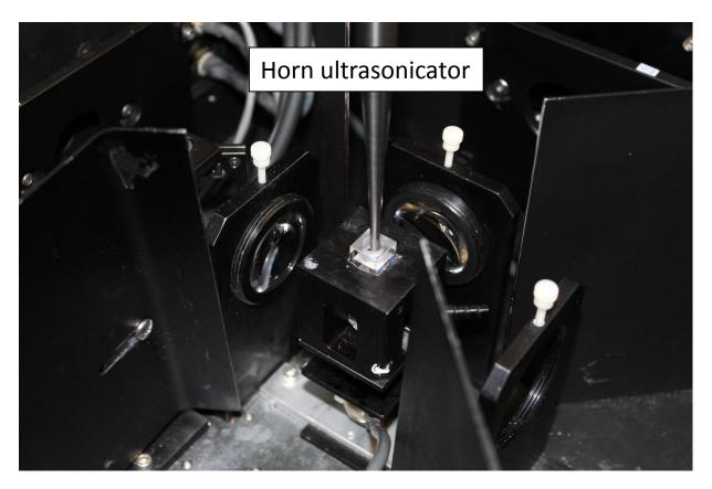
**Figure S13.** Image of experimental setup for photoluminescence studies. A horn ultrasonicator was positioned through the top port of a fluorimeter for *in situ* monitoring of the photoluminescence during ultrasonication.
