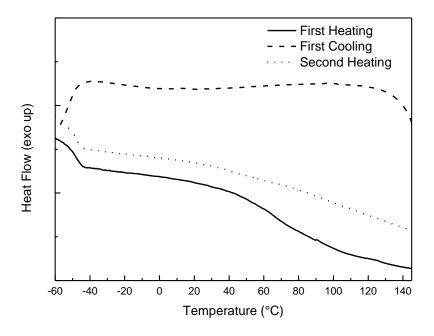
**Figure S5.** Thermal analysis of  $[Eu(BKB)_{1.5}](ClO_4)_3$ . Modulated differential scanning calorimetry (DSC) curves of  $[Eu(BKB)_{1.5}](ClO_4)_3$ ; first heating (—), first cooling (- - ) and second heating (…). The experiment was conducted with heating and cooling rates of 10° C/min under N<sub>2</sub> atmosphere.
