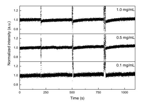
**Figure S23.** In situ monitoring of the ultrasound induced dissociation of  $[Eu(DKD)_{1.5}](NHEt_3)_3$ . Solutions of  $[Eu(DKD)_{1.5}](NHEt_3)_3$  in CHCl<sub>3</sub> (1.0, 0.5, 0.1 mg/ml) were subjected to three sonication pulses with a duration of 5, 10, and 20 sec. The samples were excited at 275 nm and the intensity of the  $Eu^{3+5}D_0 \rightarrow {}^7F_2$  emission band was monitored at 615 nm.
