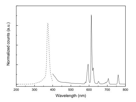
**Figure S17.** Excitation and emission spectra of model compound  $[Eu(MebipC_{12}H_{25})_3](ClO_4)_3$ in CHCl<sub>3</sub>. Excitation (- - -) and emission (—) spectra of  $[Eu(MebipC_{12}H_{25})_3](ClO_4)_3$  in CHCl<sub>3</sub> (0.30 mM). Excitation and emission spectra were recorded with detection at 615 nm and excitation at 375 nm, respectively.
