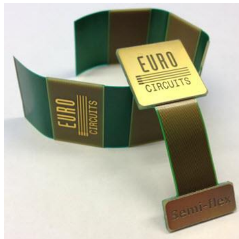
Figure 42 Euro Circuits semi-flexible PCBs [1]
