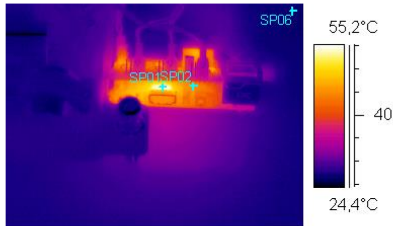
Figure 8 Processor infrared thermal acquisition with Flir camera, with measuring points. \epsilon=0.7
