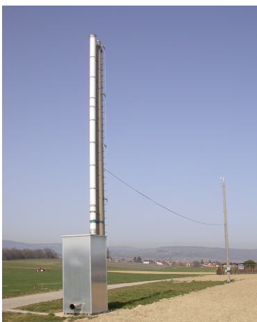
Figure 2. Rothamsted insect survey suction trap in Changins. Foreground: 12.2 m high chimney where insects and spiders are collected; chamber with suction engine and collecting pots. Background: mast with anemometer. Picture G. Blandenier.
