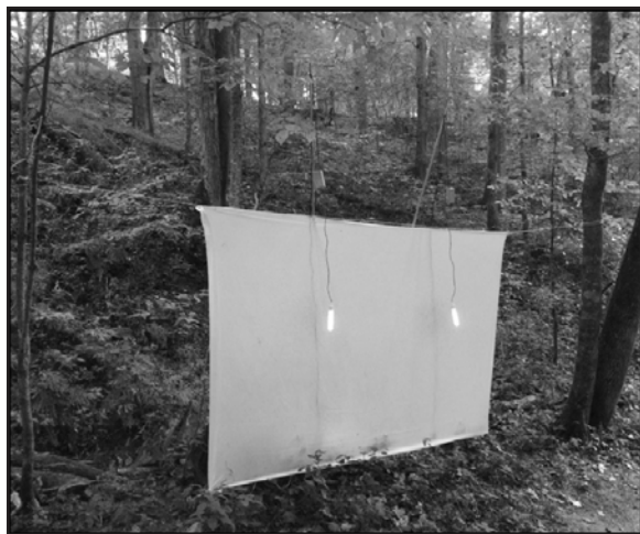
Figure 1: Cotton sheet deployed at Mammoth Cave National Park to sample Lepidoptera, illuminated by 10 w black lights with electrical harnesses.
