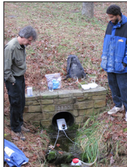
Figure 3: A National Park Service scientist and a TSU student prepare a simple dye-release system for a tracer study. (Photo taken by T. Byl, U.S. Geological Survey, 2011)
