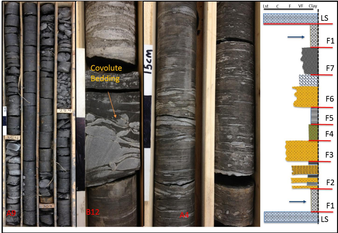
Figure 5.2. Facies 1 from the Stampede Mine. Note convolute bedding approximately 5 cm wide. Diagram on the right shows facies 1-7. Blue arrow is pointing to facies 1. The Limestone below F1 is the Beech Creek, while the limestone above is the Haney Limestone. Convolute lenses effervesce with HCl acid. Source: Imaged by the author.
