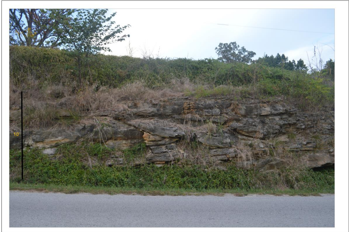
Figure 5.28. Road cut along Barren River Rd. showing facies 3. Facies 3 exhibits planar bedding that is filled with trough cross-bedded sandstone. Source: Image by the author.
