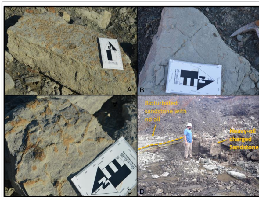
Figure 5.18. Photos from facies 6 showing ophiomorpha bioturbation (A and C), desiccation cracks (B), and bioturbated sandstone acting as a permeability barrier on top of petroleum-charged sandstone. Source: Images by the author, with all photos taken from pit A at the Stampede Mine.
