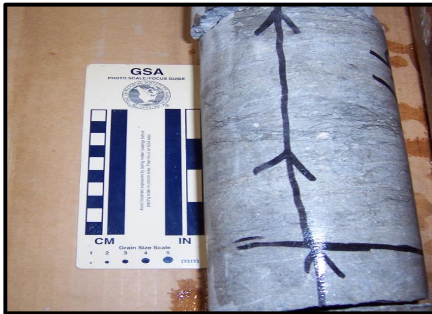
Figure 24. A cored skeletal packstone with stylolites. Core retrieved from middle of the Haney. This is an oil well with a call number of C-1167 and a well record number of #8260. This well is located in Edmonson County and has the Carter coordinates of 9-I-39 920 feet FSL, 460 feet FWL. This core was not slabbed. Arrows designate up stratigraphic sections. Source: Photographed by the author.
