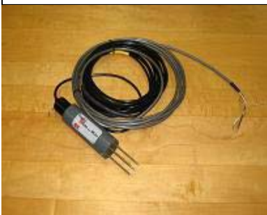
Figure 3: Probe for monitoring soil moisture levels.
