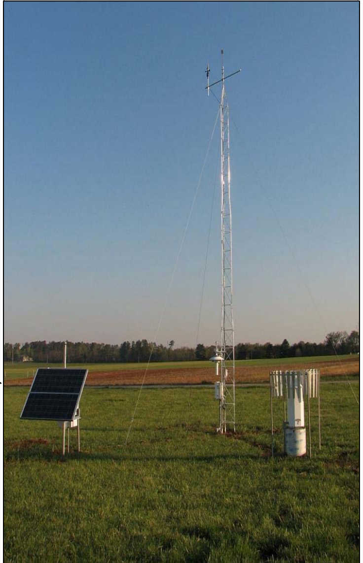
Mesonet station at the WKU farm includes a 10-meter tower with meteorological instruments, an all-weather precipitation gauge with a wind shield, and a solar panel unit to power the station.
