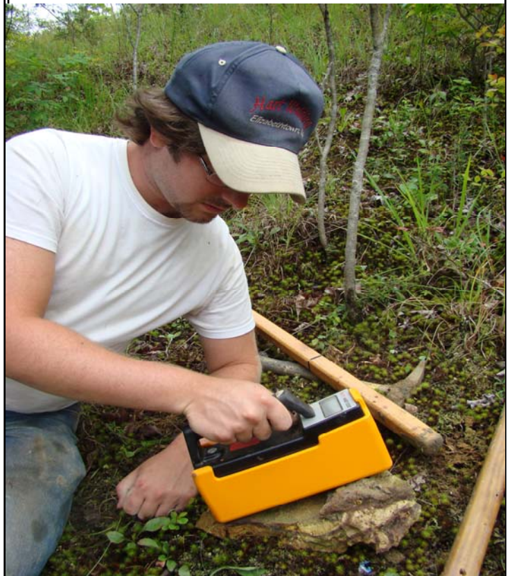
Geology student Ryan Hart taking a field measurement with the hand-held Gamma-Ray Scintillometer.
