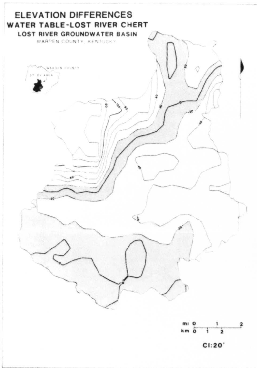
Figure 12. Contoured elevation differences between the water table and the Lost River Chert Bed. Shaded area indicates correspondence between chert and water table.
