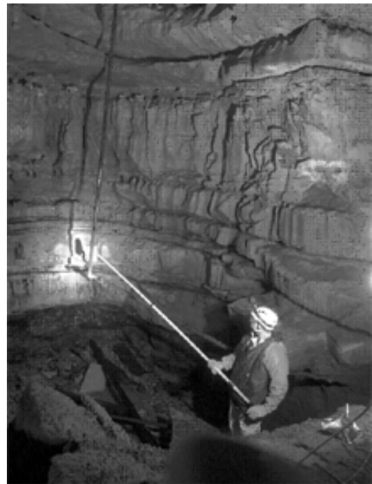
Figure 4. Water sampling at Waterfall Three using remote device to avoid a shower while sampling.
