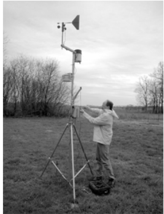
Figure 2. Weather station for recharge measurements, showing typical surface landscape above the cave system.
