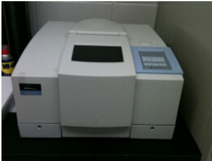
Figure 3.6. Perkin Elmer Spectrum One FTIR spectrometer.
