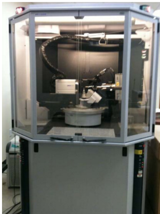
Figure 3.2. Bruker Quazar Single Crystal X-ray Diffractometer.
