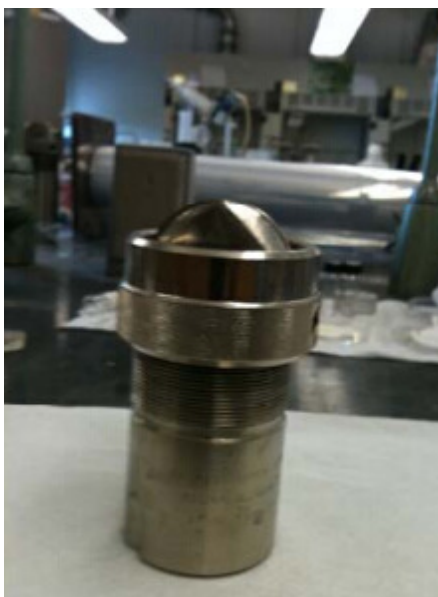
Figure 3.1 Autoclave used in the synthesis
