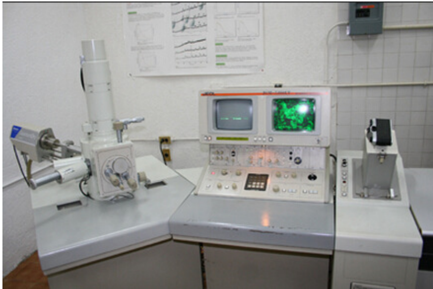
Figure 3.7. JEOL 5400LV scanning electron microscope (SEM).
