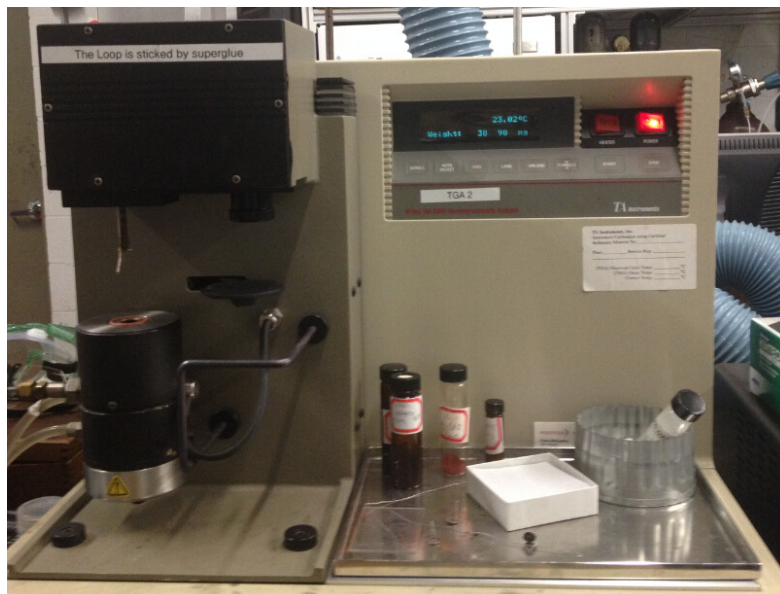
Figure 3.5. Hi-Res TGA 2950 thermal gravimetric analyzer.
