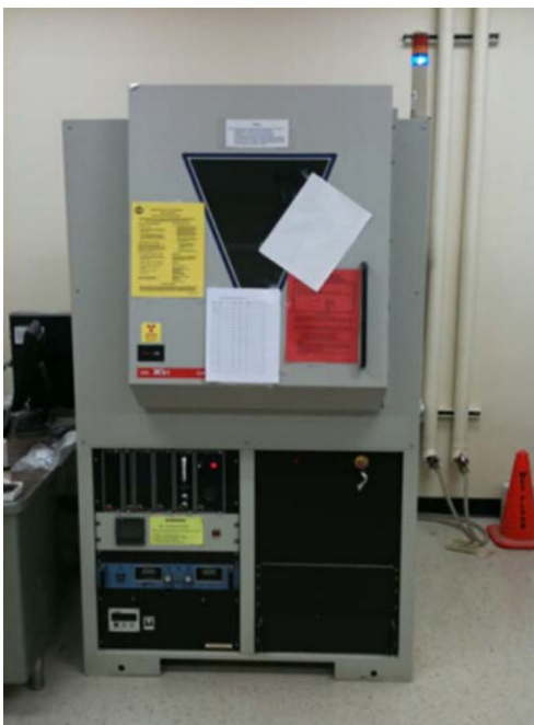
Figure 3.3. ARL Thermo Powder X-Ray Diffractometer.
