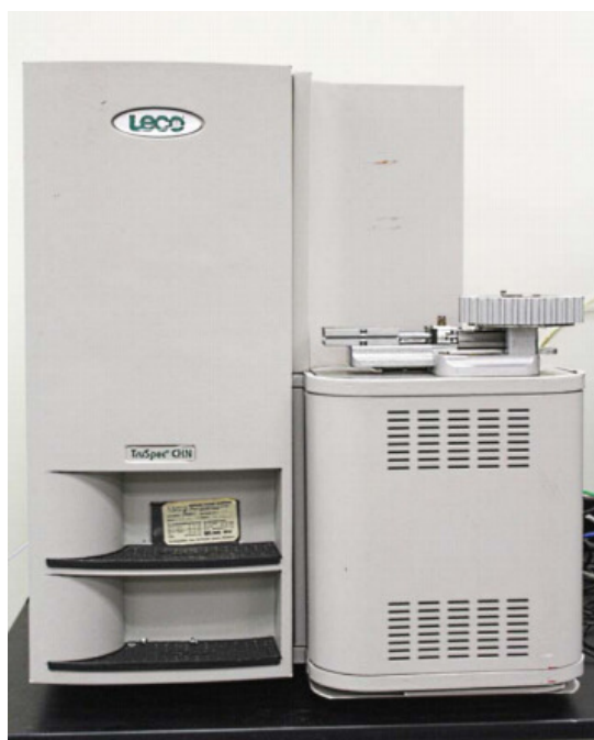
Figure 3.4. Leco True-Spec CHN Analyzer.
